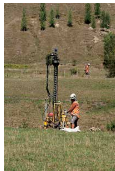
Helicopter Seismic Drilling Rig
